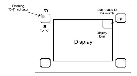
There are four control switches arranged around the display screen. Operate the switches by touching one end of the actuator onto the glass in the marked area. Keep the actuator in position until you see a change in the display or the flashing indicator.
