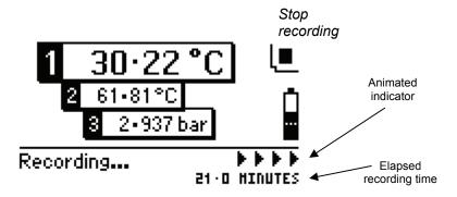
The temperature of the probes, the pressure sensor reading and the elapsed recording time are shown on the display throughout the recording run.\*
