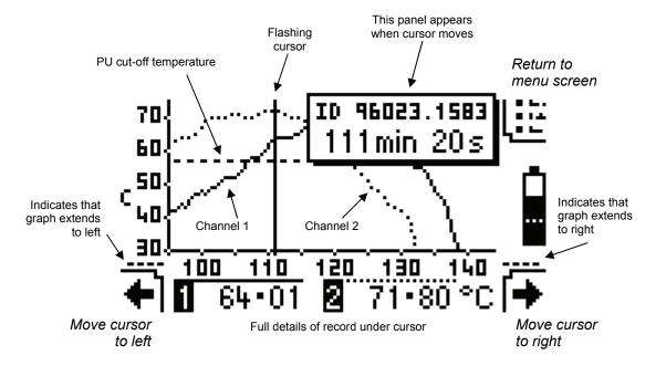
Shows the data in the recorded file as a graph. The temperature (in the selected display units) runs up the vertical axis and elapsed time (in minutes) runs along the horizontal. \*
