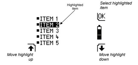
There are stages in the operation and configuration of the instrument when you need to choose an action etc. from a menu list. A menu shows all the possible choices or items in a vertical list. The method of operation is the same in every case although there can be as few as 2 and as many as 6 items in the menu list.
